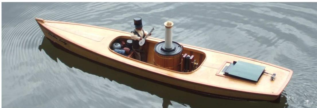
The hull is from Ebay, the boiler is made from a soup can, and the engine constructed for me by Paul, who carefully hid the electric motor at its bottom end. A dolls house figure was posed to play the banjo and fitted with a top hat. The power source is hidden in the compartment at the front of the cabin, topped by boxes barrels and a whisky jar for the banjo player.
