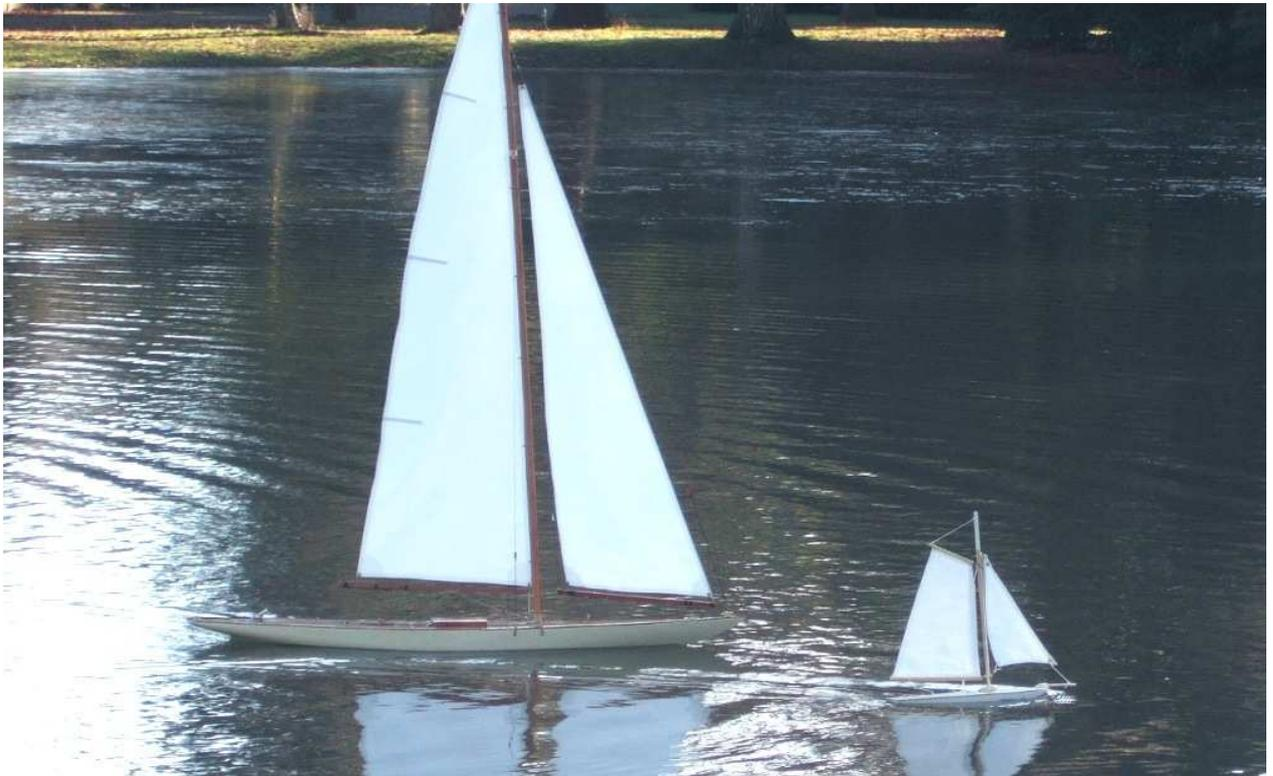
My first simple attempt at a Gaff rigged boat was to try it on an old Star Yachts hull. This too at 16 inches is a free runner, and sailed reasonably well although still needs the inevitable mods.
