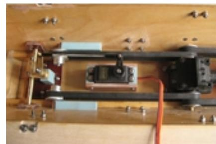
There are no seals fitted to the drive shafts or steering 'rack'; to cope with any leakage a bilge pump is fitted, this is shown on the right of the following picture with the 'jet' drives at the top & bottom left.
