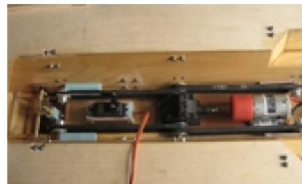
Steering is via a central servo connected to a rod sliding in a slotted tube, looking from the outside like a normal steering rack.
