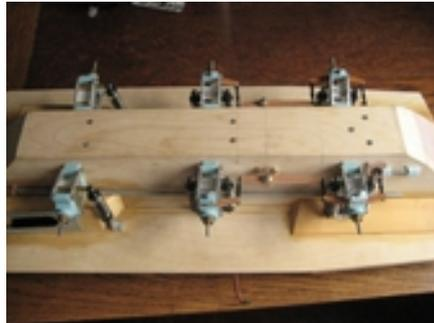
The suspension is scratch built from aluminium & various plastics. The drive shafts from brass & stainless steel. The 10 sprung shockers are 1:10 scale.
