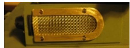
The 'Jet' drives were 'bunged up' with bits of stick, I was lucky it still worked. I made some inlet filters from brass mesh & brass plate. One is shown here before painting in olive drab.
