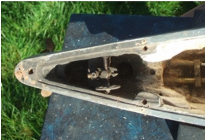
The next job will be to replace the two smaller decks, made from ply, not the thin sheet of the original which split when being removed, making them no good for reuse. Following this I will make a start on the design of the main central section of the superstructure, more about this next month.
