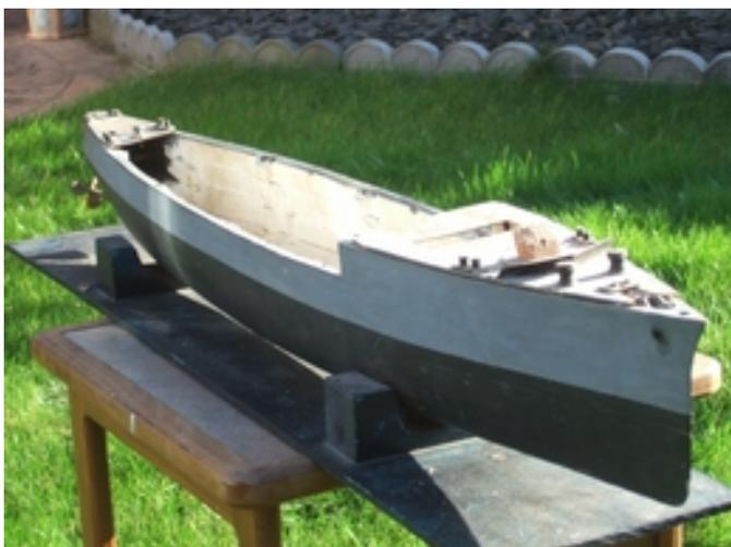
When the two decks were removed, work started on rubbing down the old paintwork, a job I was glad to see the back of, sanding down through years of over painting and creating quite a mess in the process. Now could be seen the way the engine mounting was held in place by drilling through the hull bottom and running bolts through from the outside. The repaint was just a matter of base coat, then grey and black to match the original finish.
