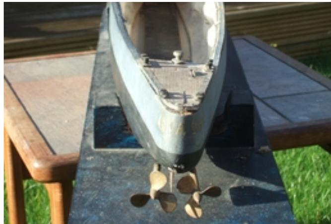
With the rear deck removed the mechanism which operated the small tab rudder could be seen, a feature which I intended to keep. I decided to leave the interior paint work, and large metal ballast weight bar as they were.
