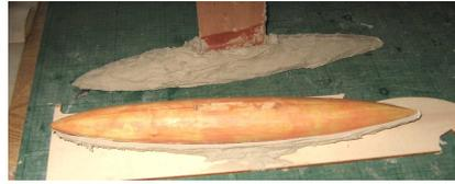
I made the mould using car body filler 'Davids Isocon', I've used this several times before and find that it works very well. Just ladle it on the pattern and smooth it as best you can; I try to get a thickness of about 5mm.
