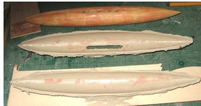
The halves are then put back together and the joint covered with Isocon to stop any leaks. After the resin filler has dried out, I left it for two days.
