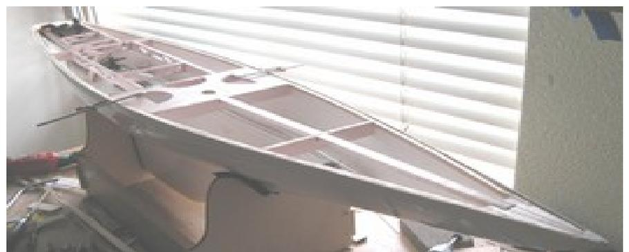
Here with the five 'G' clamps shows the under deck supports pretty well finished, It also shows the cambered cross deck beams, I had decided quite early on to have a cambered deck, the plan shows it flat but I'm not a fan, the point to remember is to pull a line from bow to stern along the centre line this gives the height you have to work to. When finished I'm sure it's an improvement.
