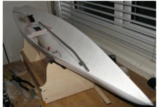
This shows the boat with the inwales fitted and the bow and stern plates fitted, the latticed deck supports as well as all the ply parts are all on one sheet and are laser cut, the cutting is very accurate but requires a lot of cleaning up, it was then painted with good old fashioned pink primer and white top coat.
