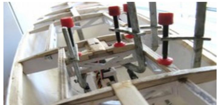
After finishing the supporting deck frame and fitting the mast tube it's time to fit the deck, my tried and trusted method is to coat the whole of the underside with thin two part resin to ensure it's waterproof then using engineering Araldite that gives plenty of time to push and pull it into the best position, stick it down and secure it with masking tape you can add more tape pulling it down harder.
