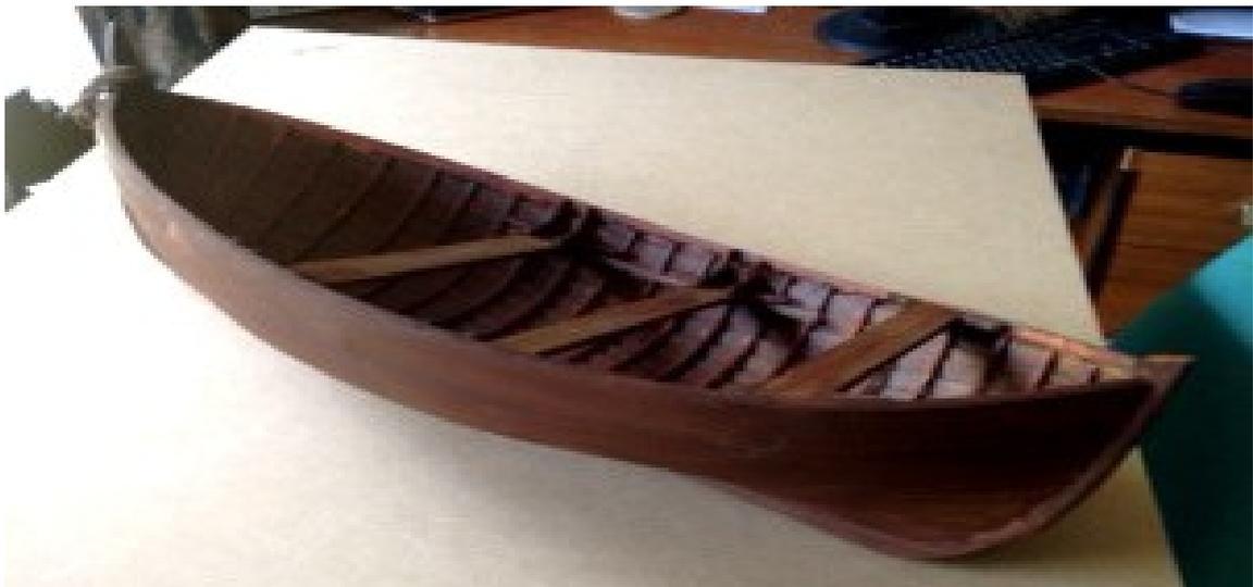
I understand that they were primarily used for catching Mackerel. In July/August a hollow was scraped out of the shingle and this was deposited in the hull where it stayed quite safely all winter and was dug out again the following year, this must have kept the planking tight.
